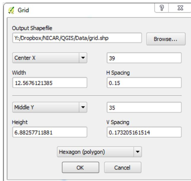
In practice, you'll need to experiment with the **H Spacing** value to produce hexagons of a suitable size. The **V spacing** value will adjust automatically. Once the shapefile has loaded, drag the points shapefile above the grid shapefile in the **Layers** panel, and you should see a screen like this, confirming that all our points are in the grid:
